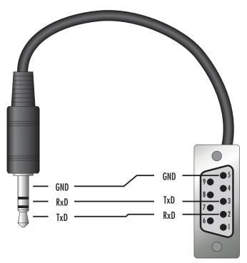
Figure 6 Serial cable wiring
