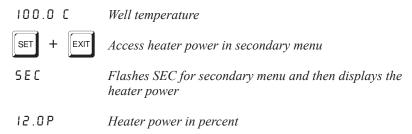
To exit out of the secondary menu press "EXIT". To continue on to the proportional band setting function press "SET".
