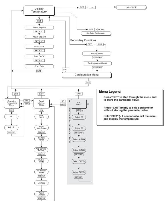
Figure 5 Controller operation flow chart
